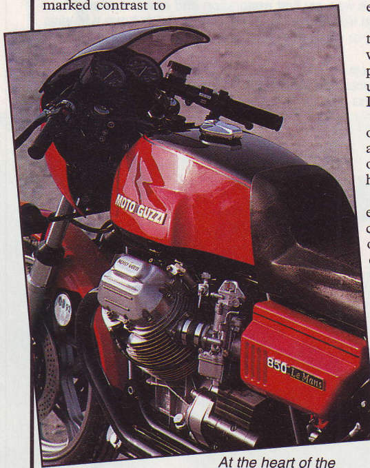
At the heart of the Le Mans is the aircooled v-twin motor.
