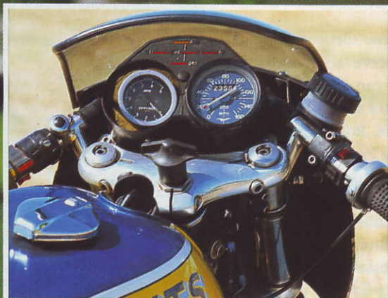
Foam mounted Smiths rev counter is accurate, speedo an ornament. Friction damper knob not connected
