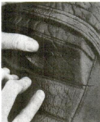
The seat developed a tear at the base of the passenger kick-up; this was not unique to just this bike.
